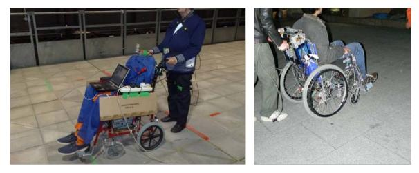
The second work stream focused on wheelchair navigation over a crossfall, or gradient across a footpath. Researchers took a detailed look at how the degree of gradient of the crossfall affects attendant pushing patterns, as well as self-propulsion patterns. Using the PAMELA
